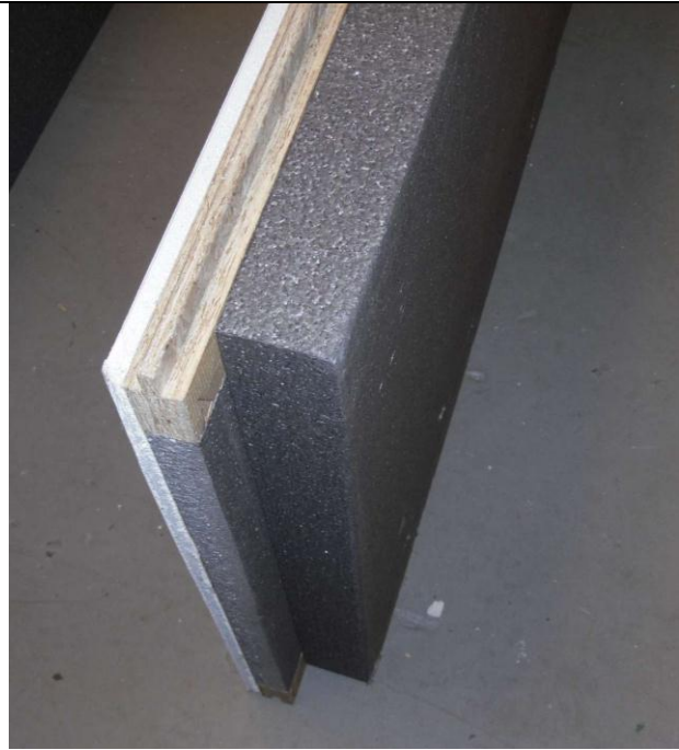
Figure 4 - Wall Assembly, Top edge
