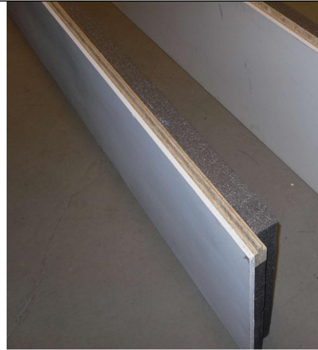
Figure 3 - Wall Assembly, Overall
