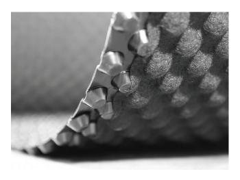
Unroll the second row and overlap the two rows where the woven backer is not present. When coming to the end of a roll and starting a second roll to finish a row, the roll width seam cannot be overlapped and should be butted together and taped using a vapour barrier rated tape.
