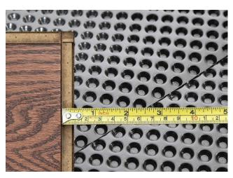
Unroll your first row with dimples facing down and lay the roll in the opposite direction that you will be installing your finished flooring product. This will reduce the odds of a floor seam falling directly on top of an underlayment seam.
