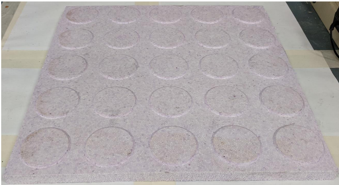
Figure 3: Specimen tested in accordance with ASTM D6364-06
