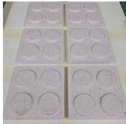
Figure 2: Four support points per specimen
